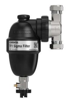
A high-performance, magnetic in-line system filter, the TF1 Sigma Filter is ideal for restricted spaces as it is capable of multiple orientations. This simple to install, composite plastic filter fits onto vertical and horizontal pipework, and works by allowing hydrocyclonic action to deliver contaminants to the unit's powerful magnet assembly for safe removal.
