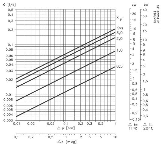
All RAS-C<sup>2</sup> Combi: capacity with P-band between 0.5K and 3K
