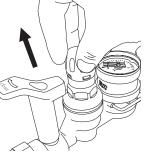
2. Turn the adjustment knob anti-clockwise to decrease the outlet pressure down to it's minimum setting.
