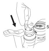
When the desired outlet pressure is reached, push the knob downwards to lock it into place and set the pressure.
