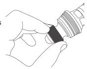
3. The strainer can easily be removed by sliding it off the end of the cartridge.
