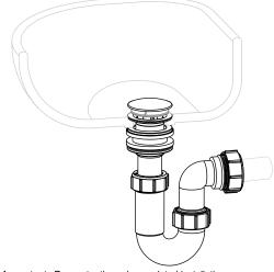
9. *Important* - Run water through completed installation, *Inspect all joints for leaks.*
