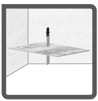
When using an upward cutting blade (jigsaw) or a circular saw, panels should be cut face down to avoid chipping.
