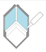
Multipanel® Seal is an all-in-one kit for sealing the bottom edge of Multipanel® at a shower tray or bath. See separate installation guide.
