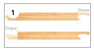
Hydrolock panels are supplied as standard with a tongued long edge and a grooved long edge. When fitting panels into an extrusion, the protruding tongued or grooved edge should be cut off.
